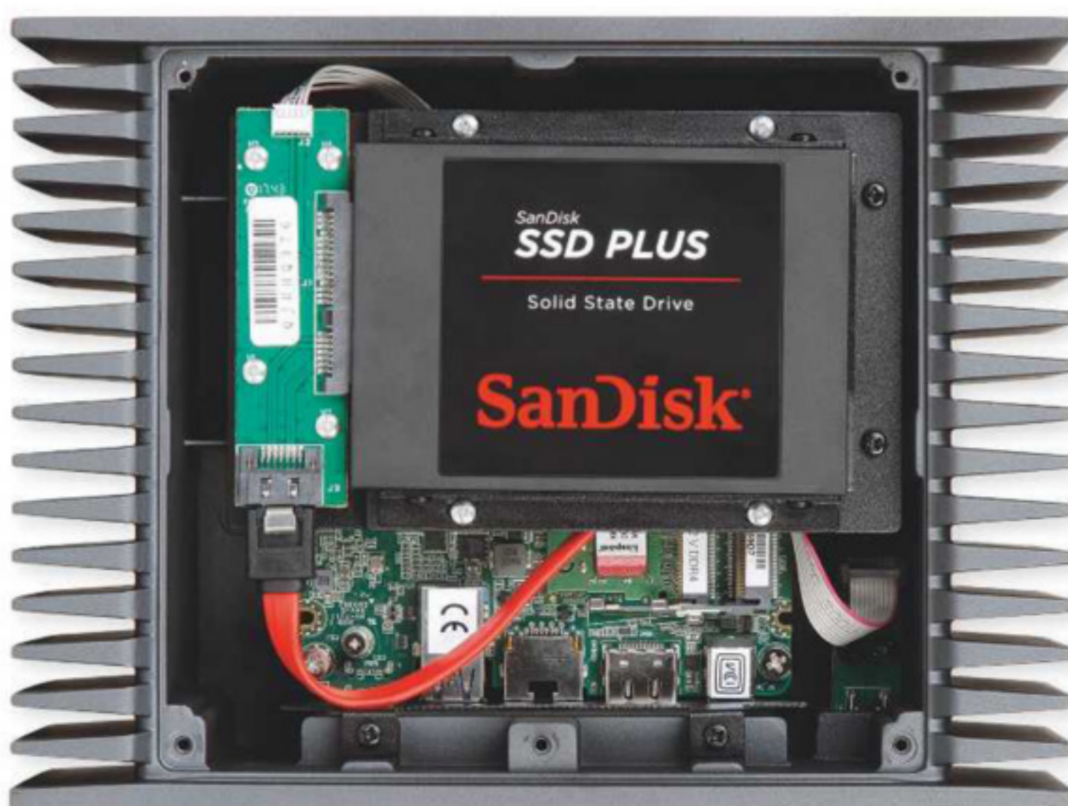
RIGHT: The Roon Nucleus+ is based on an Intel Nuc7i7BNH motherboard solution, complete with Intel Core i7 processor (running Roon's custom Linux-based operating system) and 8GB of SDRAM. A SanDisk SSD drive is fitted here
